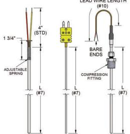
**Note:** L is the overall length of the sensor to the transition, wire, plug, head, or fixed attaching device. L excludes
