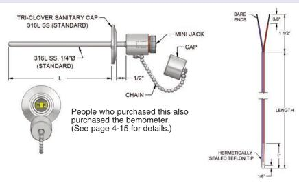
Moisture, rough handling and severe conditions all pose grave threats to the functionality of Type T thermocouple measurements - measurements which are a critical component of many high accuracy laboratory and pharmaceutical applications.
