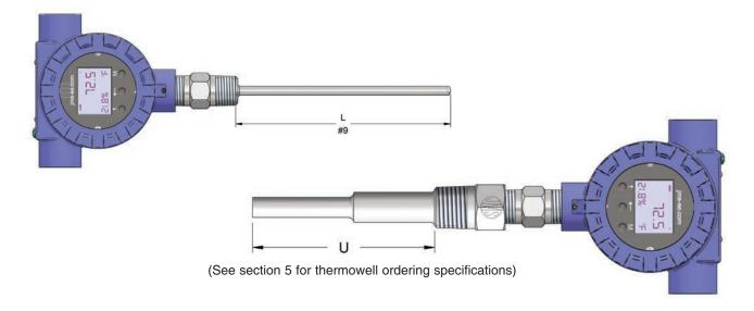
The 888 series specified with these ordering symbols include a temperature sensor assembly with an integral transmitter and indicator. The sensors are 316 stainless steel and 1/4" outside diameter. Thermocouples have ungrounded junctions. RTD's have a 3 wire configuration and a 0.00385 alpha. The most popular assembly features a spring-loaded fitting with a thermowell.
