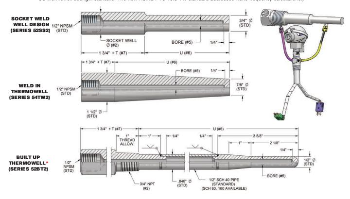
\*Design does not meet ASME PTC 19.3 TW specifications
