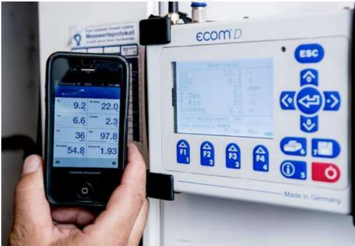
Shown here is a typical Wi-Fi configuration when the ECOM application is installed on a smart phone. Change settings remotely that provides good feedback of the sensor to the magnetically mounted hand-held unit.
